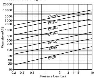
Pressure loss diagram with the valve open at 20°C. The values indicated are applicable to spring loaded valves with horizontal flow. With vertical flow, insignificant deviations occur only within the range of partial opening.
