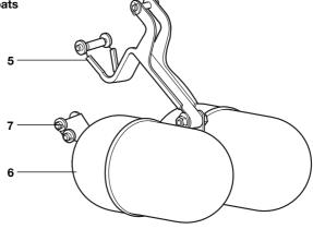
F Trap and outlet check valve mechanism
