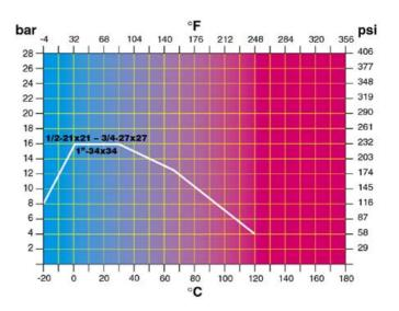
Pressure / temperature ratings 1 bar = 14,5 p.s.i.  $^{\circ}C = 5/9$  (  $^{\circ}F$ -32)  $^{\circ}F = 32+9/5$   $^{\circ}C$
