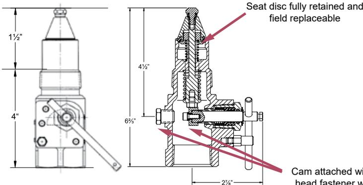
Cam attached with Allen head fastener which is accessed from the 1/4" pipe plug on side of the body
